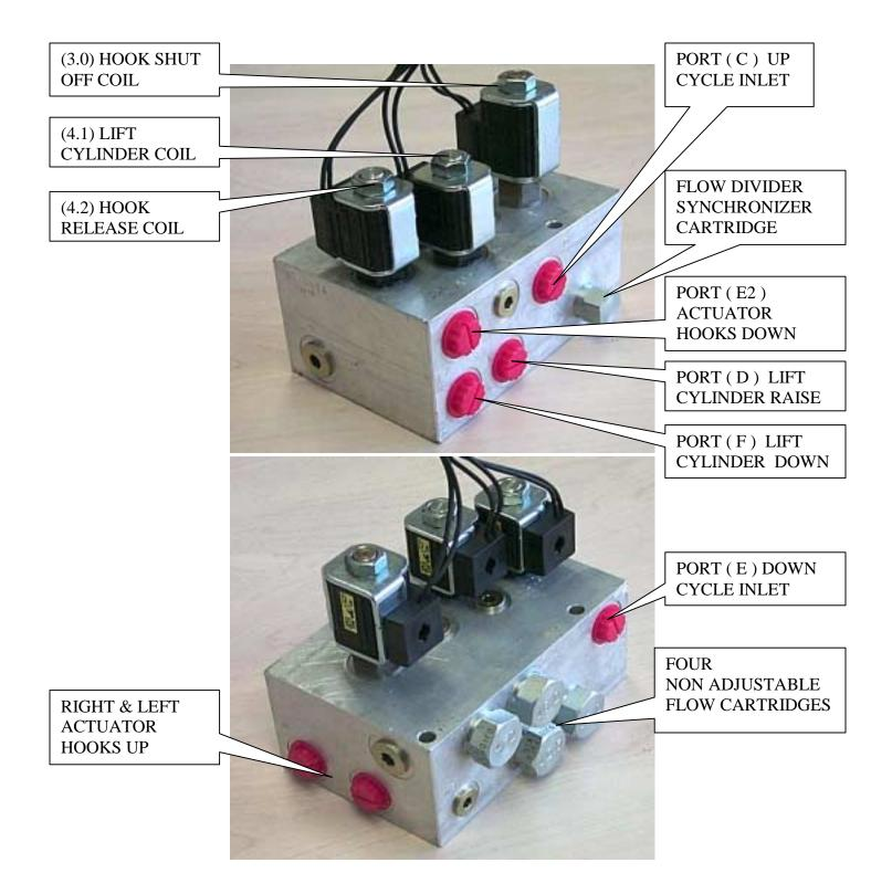
NOTE: PORT AND COIL LOCATIONS ARE STAMPED IN MANIFOLD HOUSING
